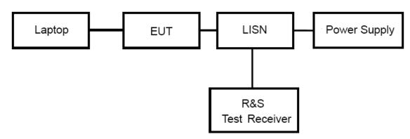
Note: Power Supply is AC Power source and it is used to change the voltage 120V/60Hz.
