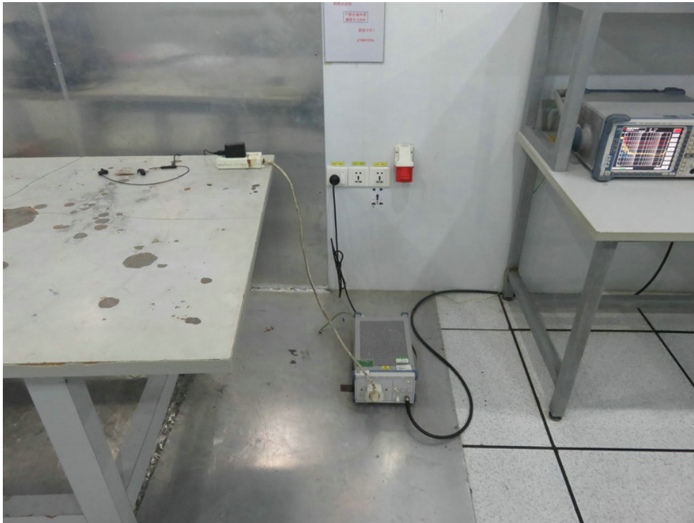
Photo of Conducted Emission Measurement
