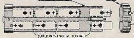
Figure 3. Battery Case, Showing Correct Method for Installing Batteries.
