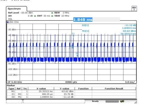
The resulting plot data was extracted and post processed, giving a duty cycle of 21.98%.
