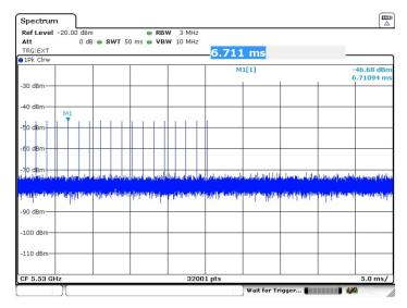
Peak of -46.68dBm, with losses at combiners factoring antenna gain to be 15.81dB, therefore level going into antenna port is -62.49dBm which exceeds threshold level of -64dBm for successful detection.
