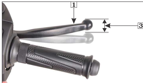
(1) Front brake lever (3) Free play: 10-20 mm
