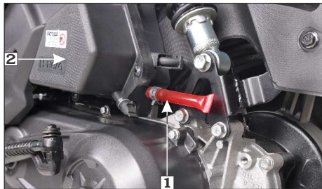
(1) Drain tube (2) Air cleaner assembly
