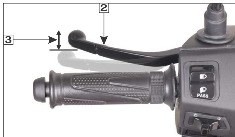
(1) Integrated brake lever (3) Free play: 10-20 mm
