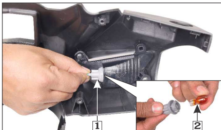
(1) Front turn signal lamp holder (2) Bulb
