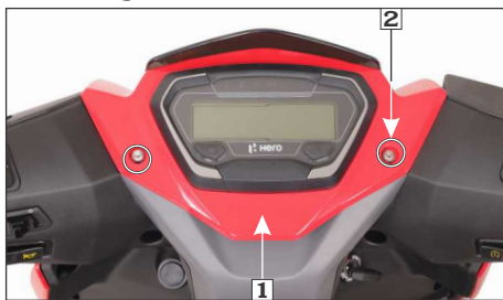
(1) Top handlebar cover (2) Allen screws
