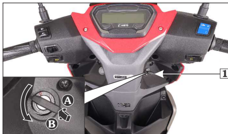
(1) Ignition key (A) Push in (B) Turn to lock
