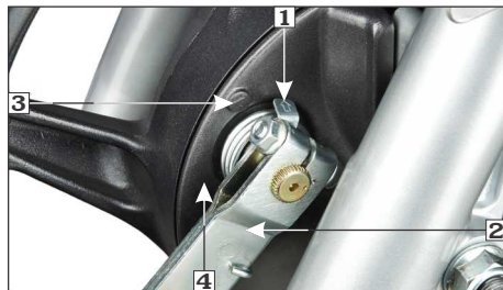
(1) Arrow (2) Integrated brake arm (3) Reference mark (4) Brake panel
