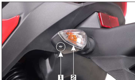
(1) Screw (2) Turn signal lamp lens
