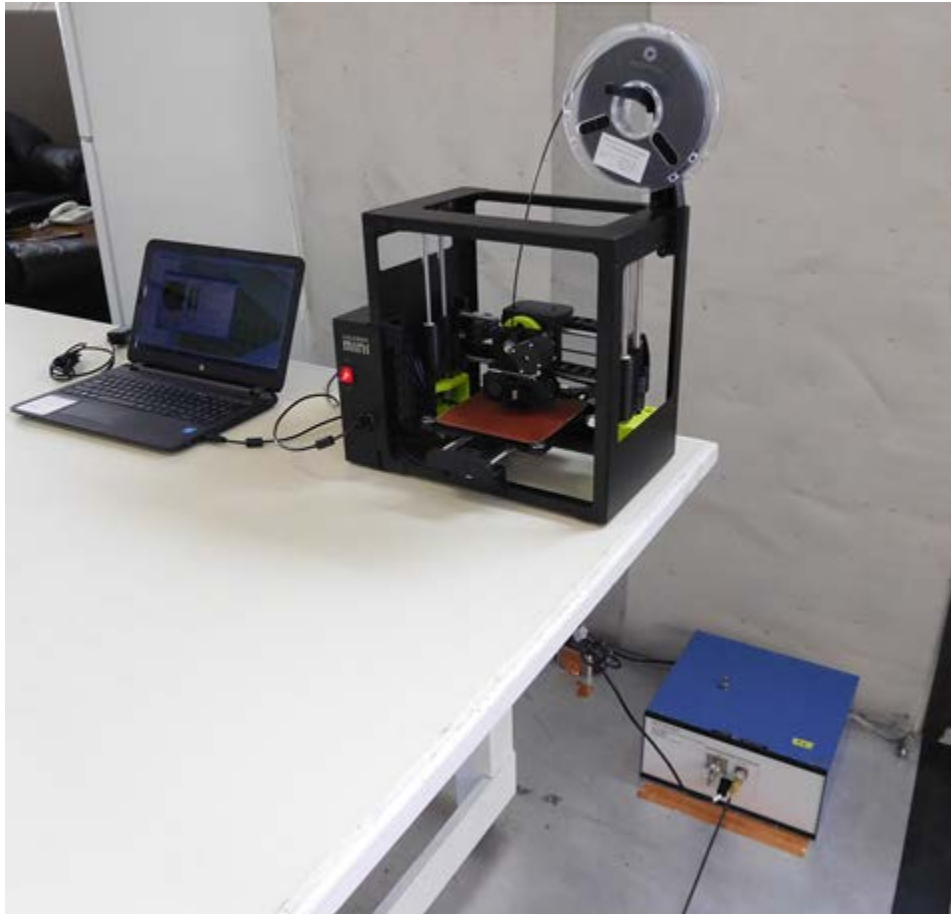
Conducted emissions test setup
