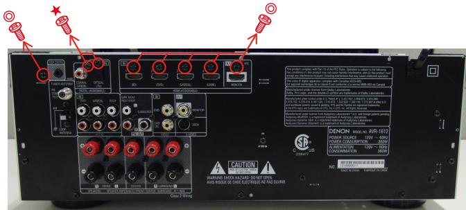
(2) Disconnect the connector board.
