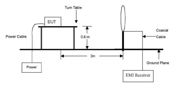
The diagram below shows the test setup that is utilized to make the measurements for emission from 30 Mb to 135.6 Mb Emissions.
