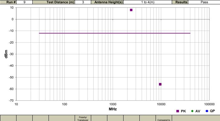
Transducer Type Compared to Spec. Azimuth Detector EIRP EIRP Spec. Limit Comments (MHz) (meters) (Watts) (dBm) (dBm) (dB) 265.0 Low Channel, 1MHz RBW 9609.080 2.5 Horz 2.55E-09 -55.9 -12.1 -43.8 PK 9609.080 2.5 270.0 Vert 2.50E-09 -56.0 -12.1 -43.9 Low Channel, 1MHz RBW 2402.317 2.5 273.0 Horz PK 6.23E-03 7.9 N/A N/A Fundamental Reference All other Out of Band frequencies greater than -40 dBc from fundamental
