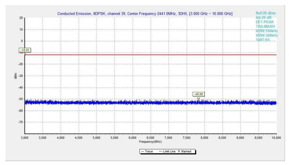
Fig.57. Conducted spurious emission: 8DPSK, Channel 39, 3GHz - 10GHz
