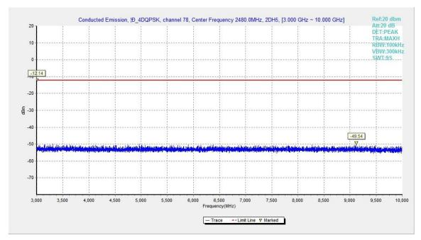
Fig.47. Conducted spurious emission: π/4 DQPSK, Channel 78, 3GHz - 10GHz
