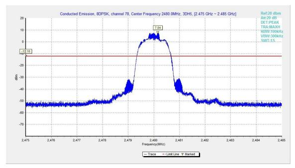
Fig.59. Conducted spurious emission: 8DPSK, Channel 78, 2480MHz
