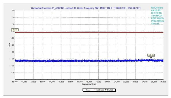
Fig.43. Conducted spurious emission: π/4 DQPSK, Channel 39, 10GHz – 26GHz
