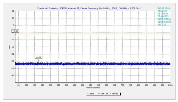
Fig.55. Conducted spurious emission: 8DPSK, Channel 39, 30MHz - 1GHz
