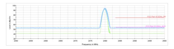
Fig.16. Frequency Band Edges:  $\pi/4$  DQPSK, Channel 78, Hopping Off, 2.38 GHz - 2.45GHz
