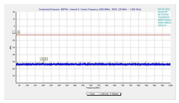
Fig.50. Conducted spurious emission: 8DPSK, Channel 0, 30MHz - 1GHz
