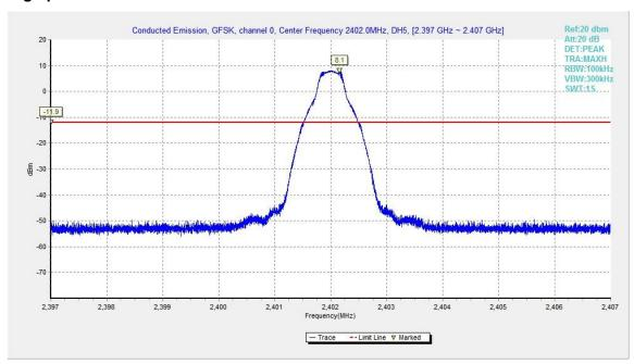
Fig.19. Conducted spurious emission: GFSK, Channel 0,2402MHz
