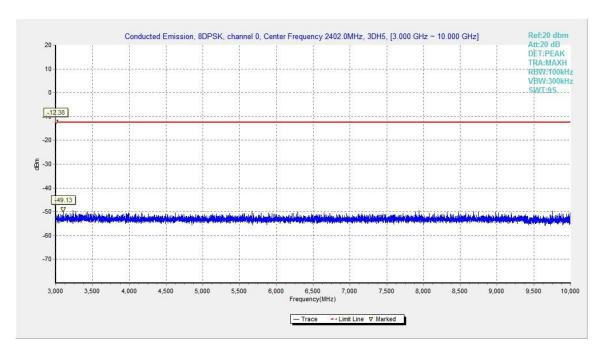
Fig.52. Conducted spurious emission: 8DPSK, Channel 0, 3GHz - 10GHz
