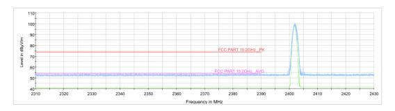
Fig.15. Frequency Band Edges:  $\pi/4$  DQPSK, Channel 0, Hopping Off, 2.38 GHz - 2.45GHz
