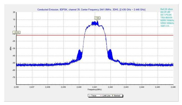
Fig.54. Conducted spurious emission: 8DPSK, Channel 39, 2441MHz
