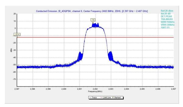
Fig.34. Conducted spurious emission:  $\pi/4$  DQPSK, Channel 0,2402MHz
