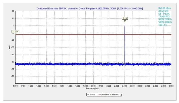
Fig.51. Conducted spurious emission: 8DPSK, Channel 0, 1GHz - 3GHz
