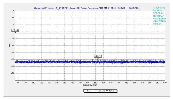
Fig.45. Conducted spurious emission: π/4 DQPSK, Channel 78, 30MHz - 1GHz
