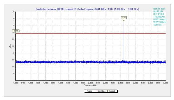
Fig.56. Conducted spurious emission: 8DPSK, Channel 39, 1GHz - 3GHz
