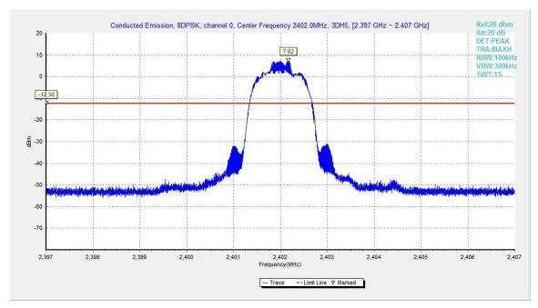
Fig.49. Conducted spurious emission: 8DPSK, Channel 0,2402MHz
