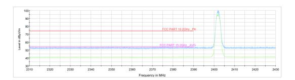
Fig.17. Frequency Band Edges: 8DPSK, Channel 0, 2.38 GHz - 2.45GHz
