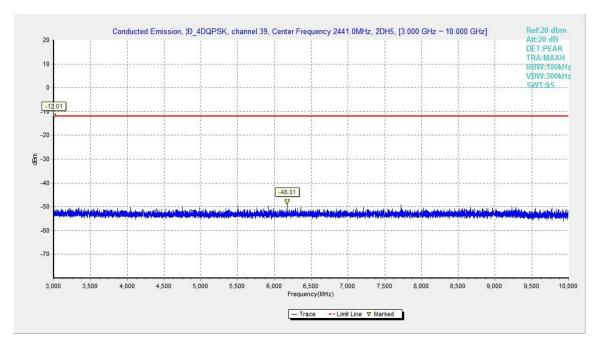
Fig.42. Conducted spurious emission: π/4 DQPSK, Channel 39, 3GHz - 10GHz
