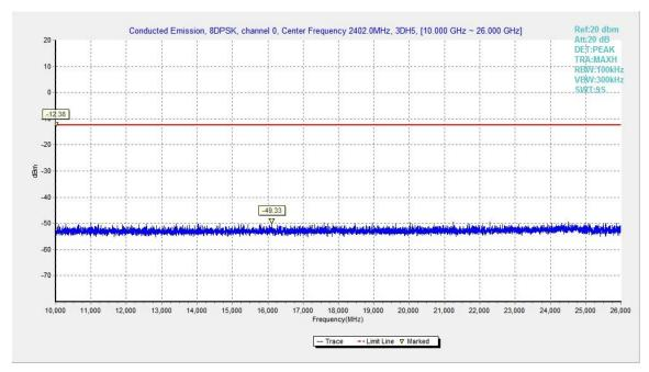
Fig.53. Conducted spurious emission: 8DPSK, Channel 0,10GHz - 26GHz
