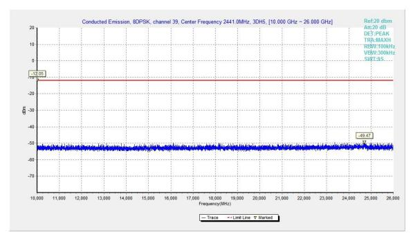
Fig.58. Conducted spurious emission: 8DPSK, Channel 39, 10GHz – 26GHz
