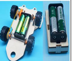
21:Install rubber band.Make sure the rubber band is attached to both pulleys.
