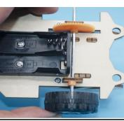
step16: Install an orange kit and a white pulley.
