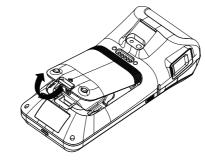
4. Put the battery door back. Press the ON/OFF key
