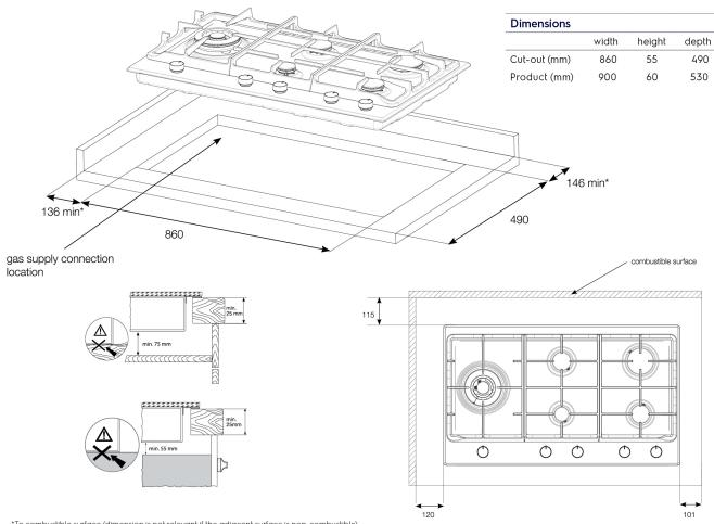
$<sup>{}^\</sup>star \text{To combustible surface (dimension is not relevant if the adjacent surface is non-combustible)}.$
