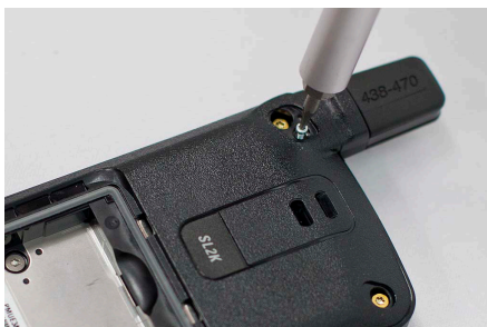
Figure 54: Antenna Screw Reassembly
