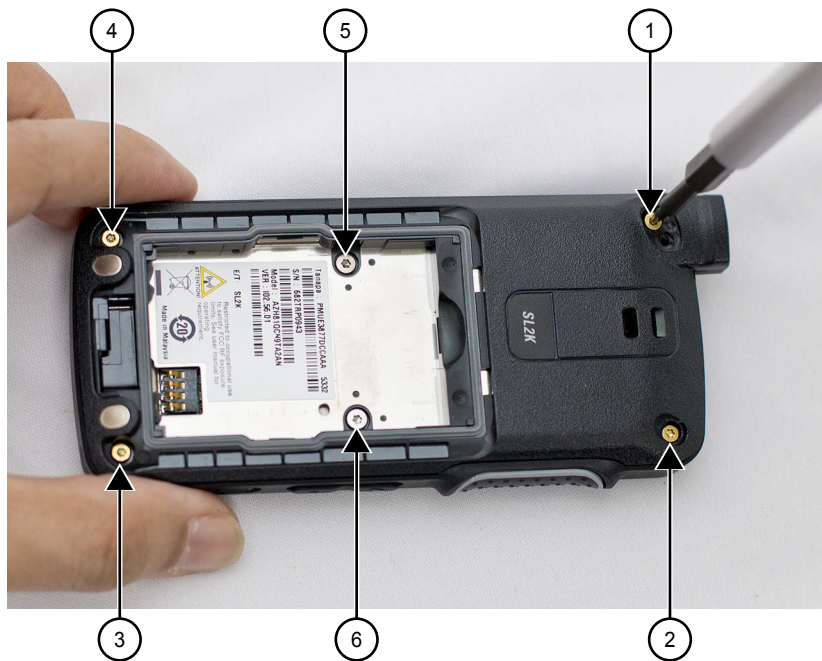
Figure 18: Corner screws and middle screws removal
