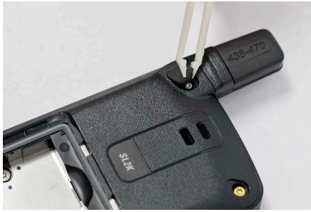
Figure 56: New Escutcheon Cover Reassembly
