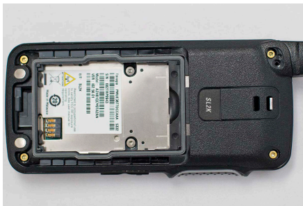
Figure 49: Screws Reassembly Completed
