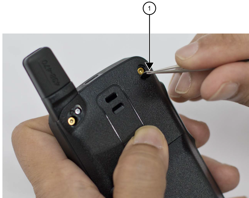
Figure 12: Escutcheon cover removal with tweezers
