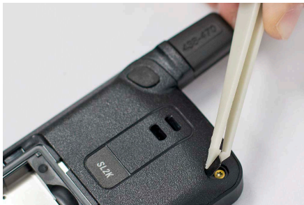
Figure 56: New Escutcheon Cover Reassembly
