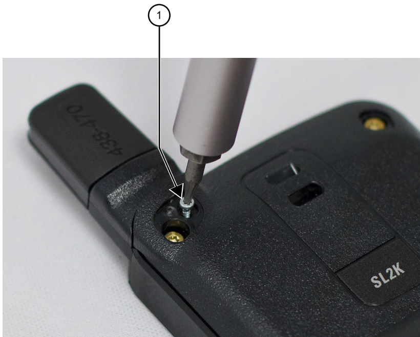
Figure 13: Antenna screw removal
