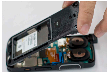
Figure 47: Back Housing Reassembly
