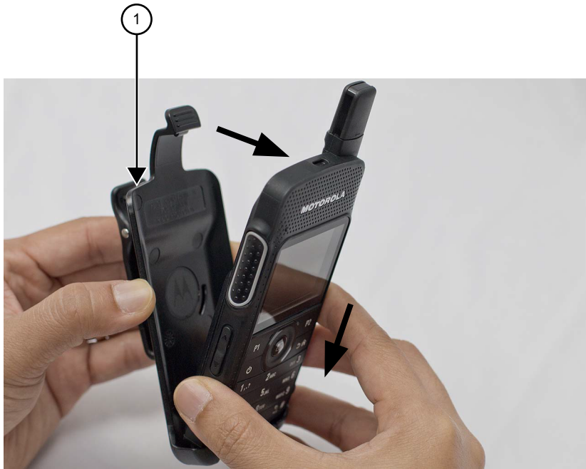
Figure 57: Refixation de l'étui
