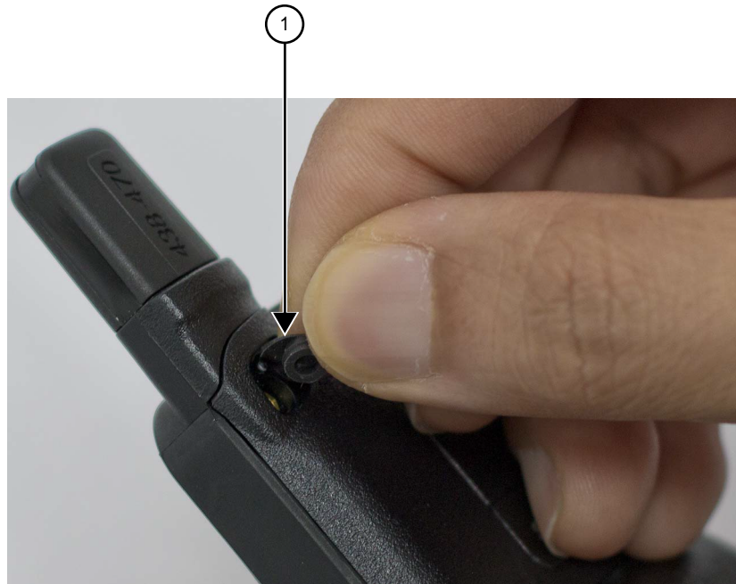
Figure 11: Antenna plug removal with fingers
