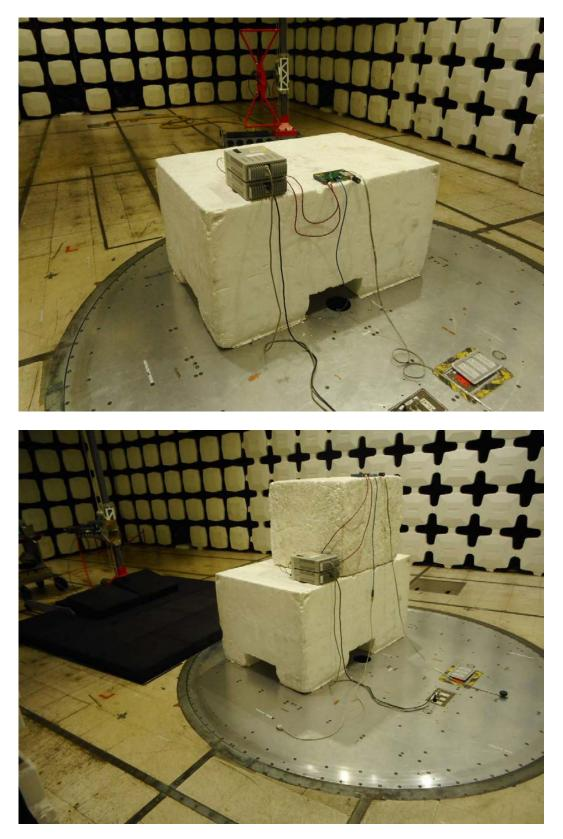
Radiated Emissions Test Configuration Photographs
