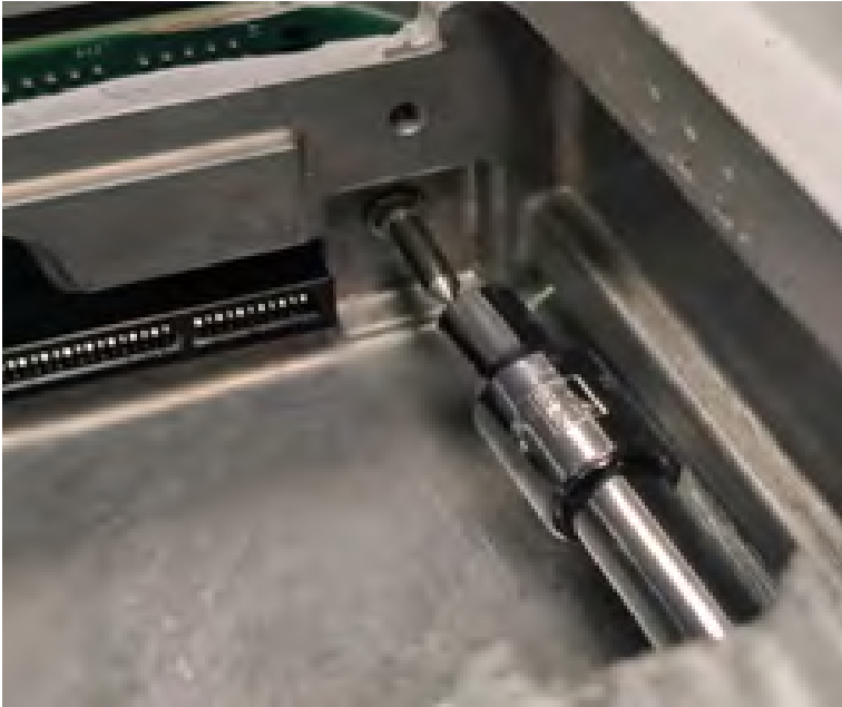
Figure 57 Removing the alignment guide pin
