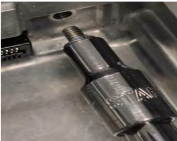
Figure 58 Alignment guide pin removed
