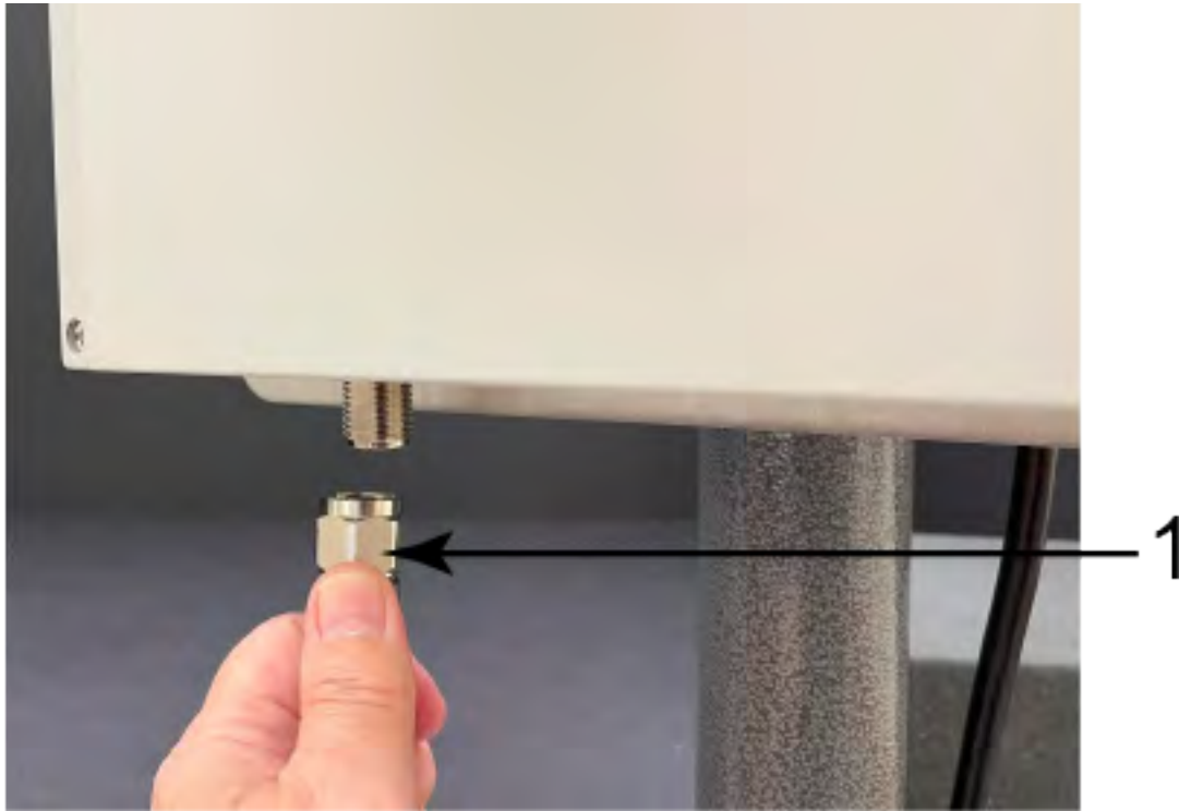
Figure 54 RF filter to IRM-STAR/IRM-MESH connection - Bottom
