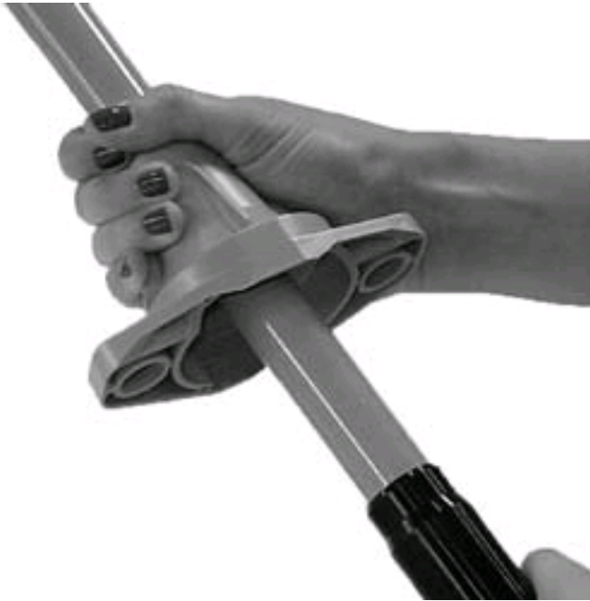
Figure 29 Remote antenna holder over the silicone
