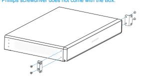
2 Slide the Box into the cabinet and insert screws through the mounting ears to hold the Box in place.
