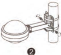
1. Secure the mounting plate to the vertical pole by threading two clamps through the mounting plate.
