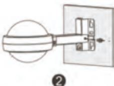
1. Secure the mounting plate on the wall using expansion bolts.
