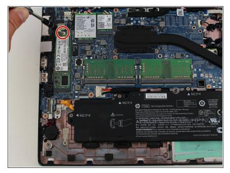
• Using a Phillips #1 screwdriver, remove the single 2mm screw that holds the SSD storage in place.
