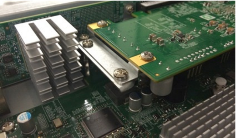
Figure 6-10. Installing the Internal Expansion Card
