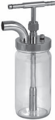
3-jet Collision Aerosol Nebulizer with direct connections to cylinder Part #19-N
