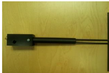
Figure 1 – MVG COMOSAR Validation Dipole
