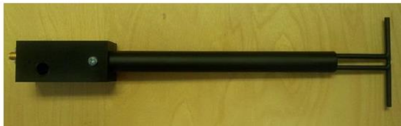
Figure 1 – MVG COMOSAR Validation Dipole
