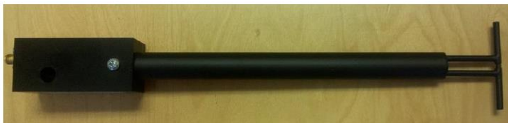
Figure 1 – MVG COMOSAR Validation Dipole
