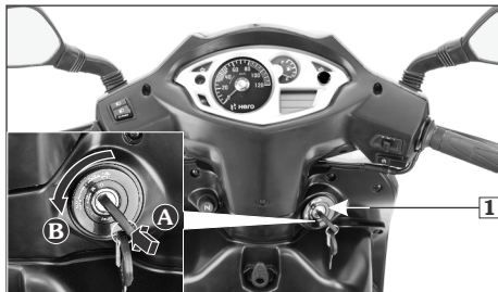
(1) Ignition switch (A) Push in (B) Turn to lock
