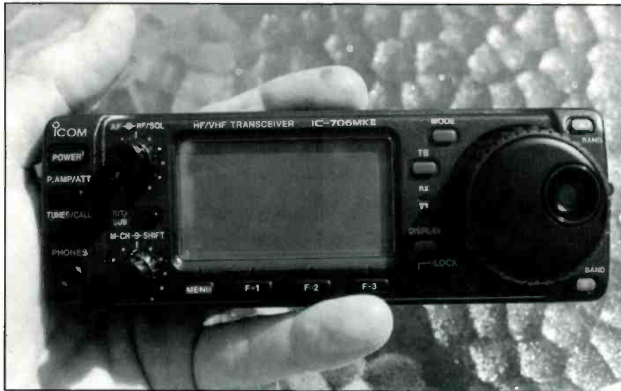
A top-notch motorcycle communications set-up has a detachable head and much-improved scanning capabilities on VHF.
