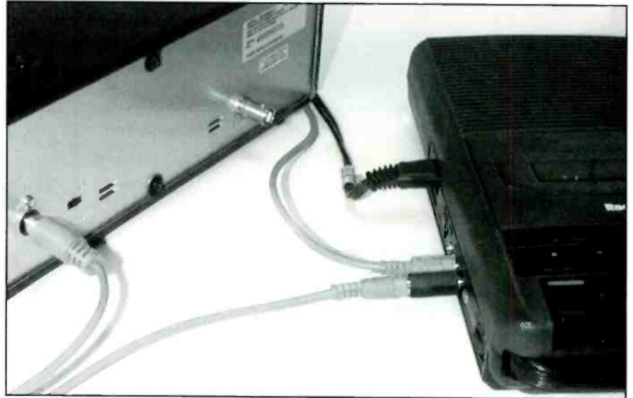
The BC-9000 XLT is one of few radios with an auxiliary control port for the recorder. The AUX from the radio is connected (with appropriate cables and adapters from RadioShack) to the REM jack of the recorder. Note that the LINE OUT jack on the Bearcat series is on the front panel.
