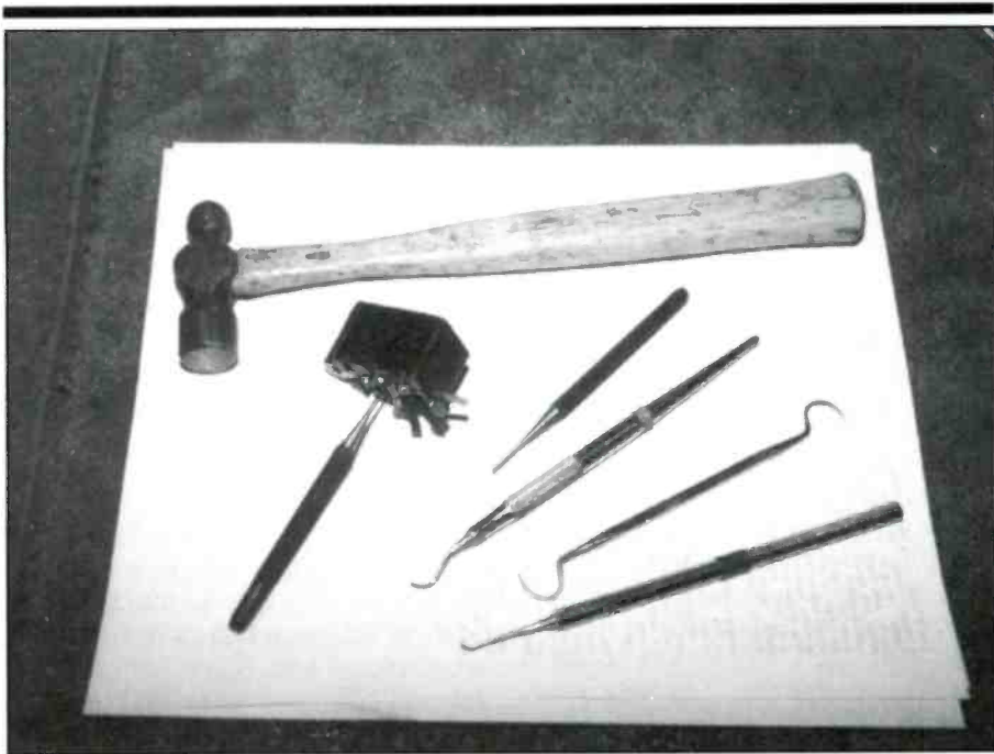
Tools of the trade for successfully rebuilding the Philco block capacitors: 1/16 inch drift pinches, a 4 oz. hammer, and dental tools. Your dentist can supply you with worn instruments on your next visit.
