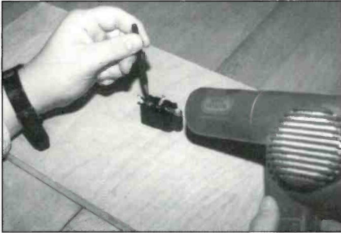
My son Tom shows how he is testing the capacitor for release with the drift punch while applying heat from a hairdryer. This is easy to do while the capacitor is installed on the chassis.
