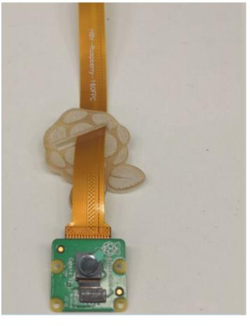
Figure 3-6 Installing the fixing film
