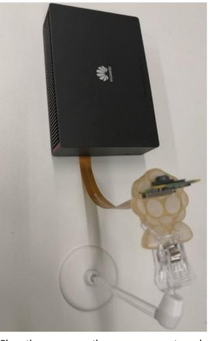
Figure 3-9 Installing the camera support
