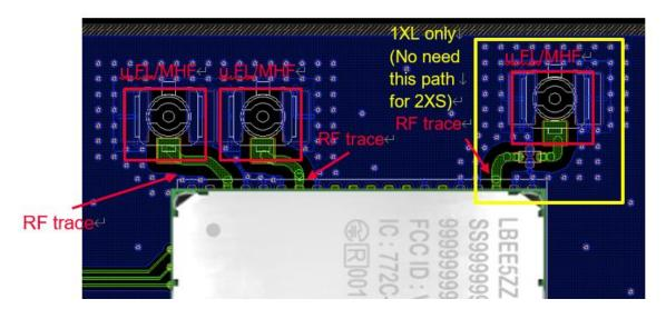
The 50ohm microstrip line needs to be copied when module is installed in the End product.
