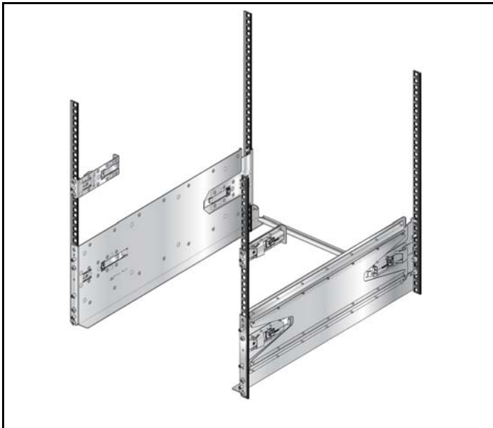
Figure 12: Both Switch Shelves Installed
