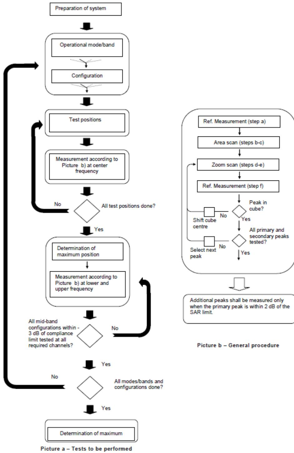
Picture a – Tests to be performed
