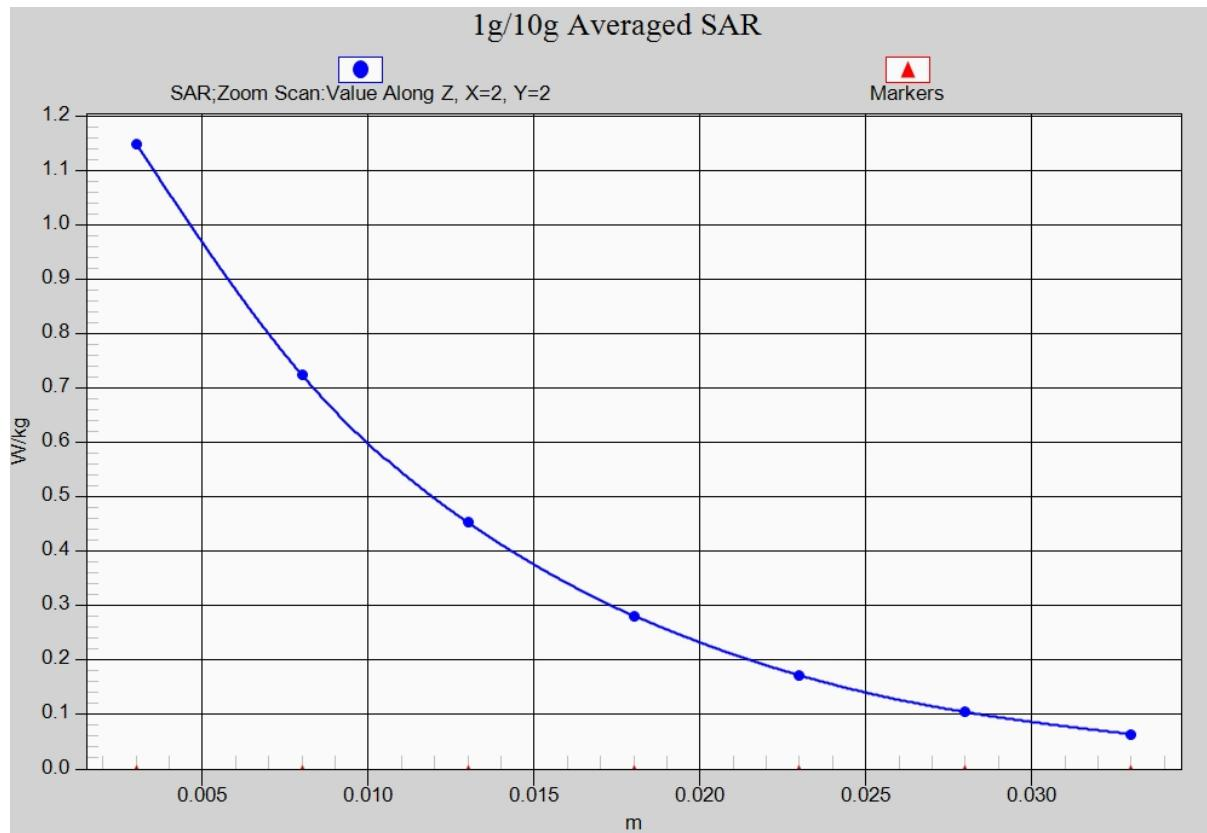
Fig.4-1 Z-Scan at power reference point (1900 MHz)
