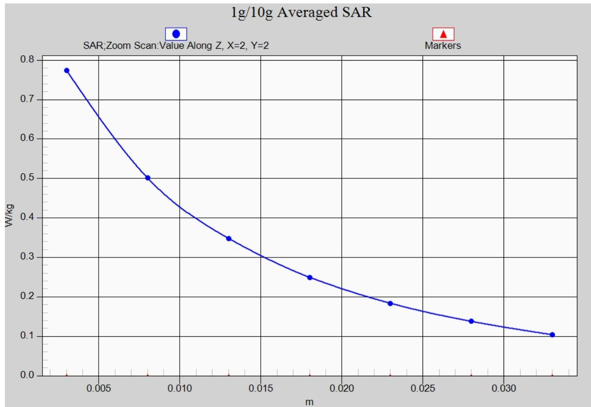
**Fig. 1-1 Z-Scan at power reference point (850 MHz)**
