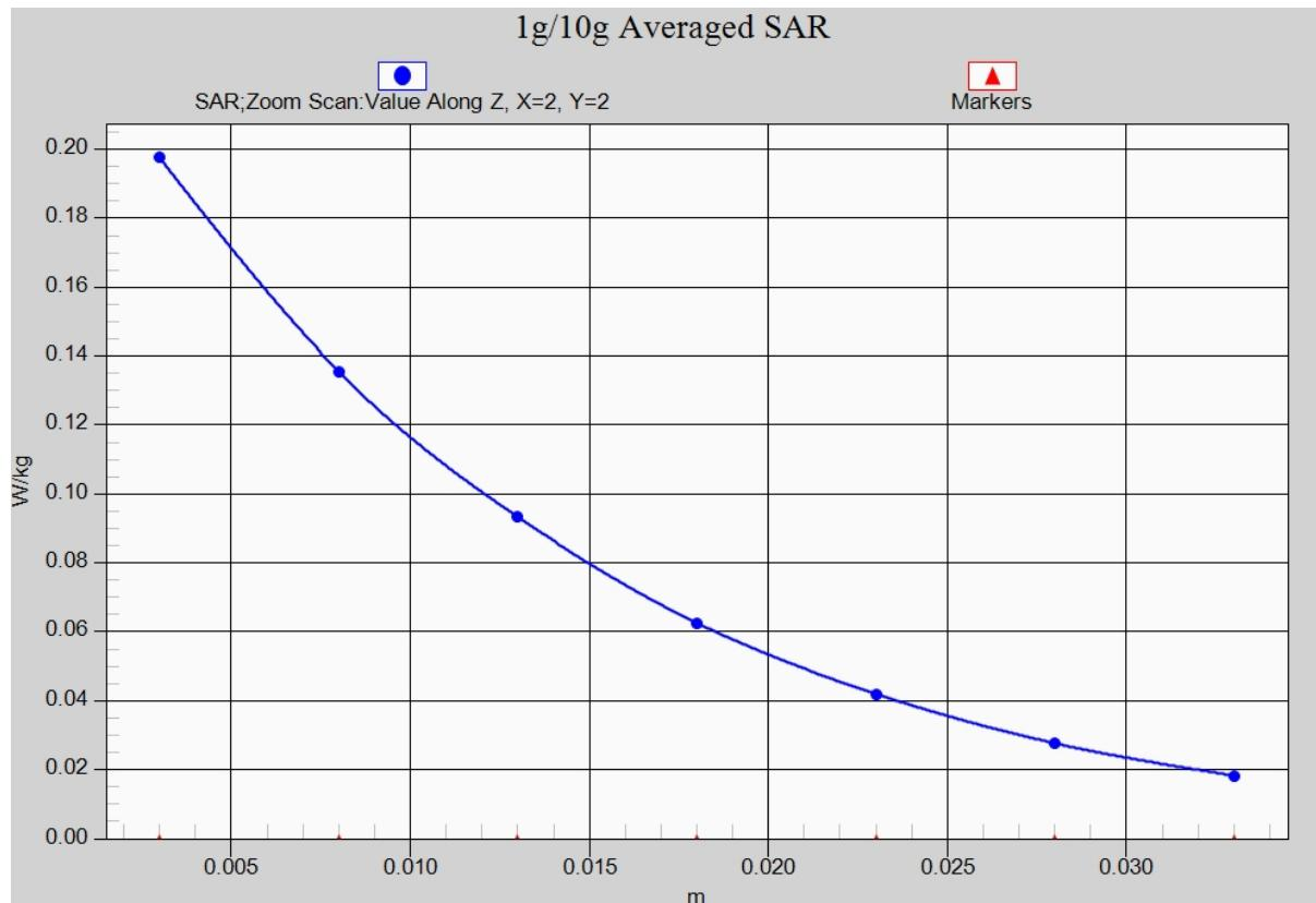
Fig. 3-1 Z-Scan at power reference point (1900 MHz)
