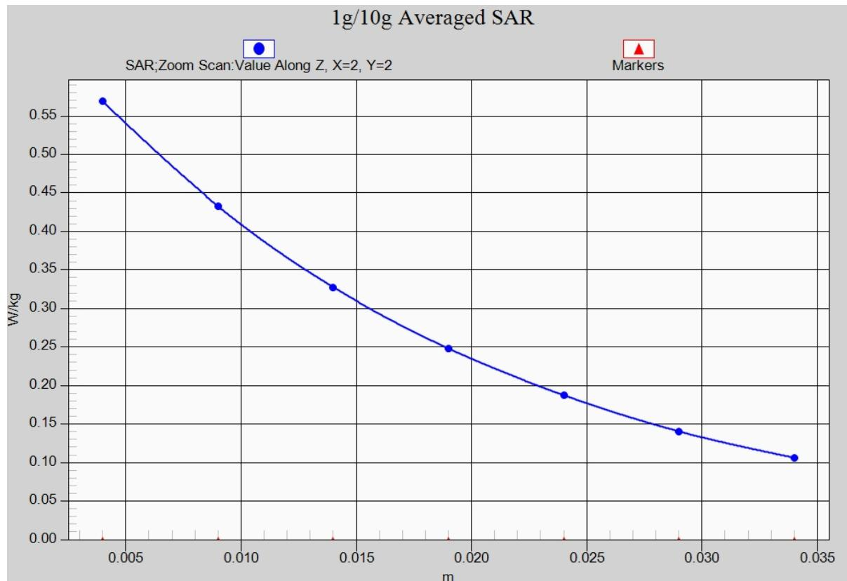
Fig. 6-1 Z-Scan at power reference point (WCDMA850)
