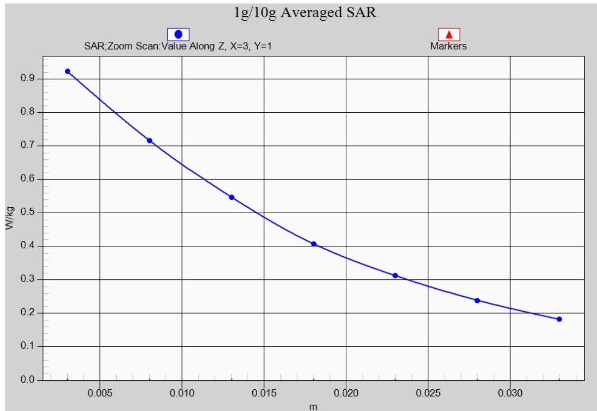
**Fig. 2-1 Z-Scan at power reference point (850 MHz)**
