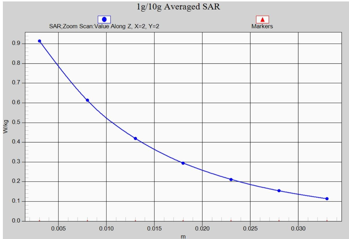
Fig. 5-1 Z-Scan at power reference point (WCDMA 850)
