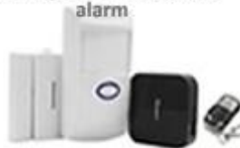
RF Bridge 433 + PIR, dvere alarm
