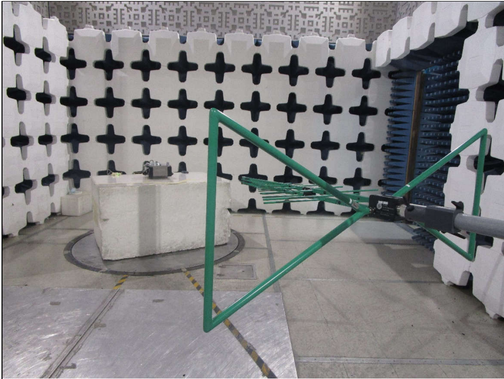
Test Setup for Spurious Emissions: 30MHz to 1GHz, Horizontal Polarization
