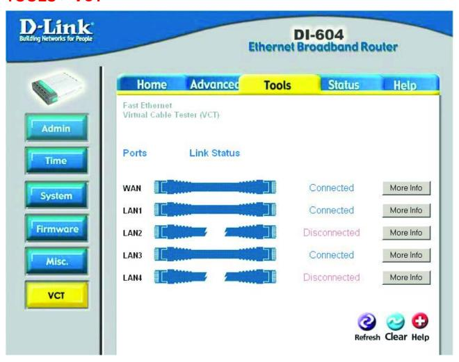
Virtual Cable Tester (VCT) is an advanced feature that integrates a LAN cable tester on every Ethernet port on the router. Through the graphical user interface (GUI), VCT can be used to remotely diagnose and report cable faults such as opens, shorts, swaps, and impedance mismatch. The VCT feature significantly reduces service calls and returns by allowing users to easily troubleshoot their cable connections.
