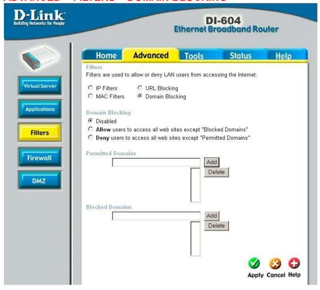
**Domain Blocking** is used to allow or deny LAN computers from accessing specific domains on the Internet. Domain blocking will deny all requests to a specific domain such as http and ftp. It can also allow computers to access specific sites and deny all other sites.
