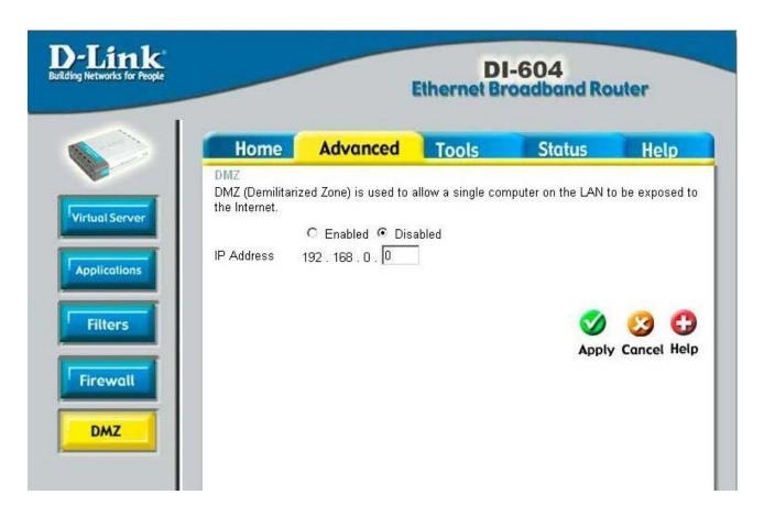
If you have a client PC that cannot run Internet applications properly from behind the DI-604, then you can set the client up to unrestricted Internet access. It allows a computer to be exposed to the Internet. This feature is useful for gaming purposes. Enter the IP address of the internal computer that will be the DMZ host. Adding a client to the DMZ (Demilitarized Zone) may expose your local network to a variety of security risks, so only use this option as a last resort.
