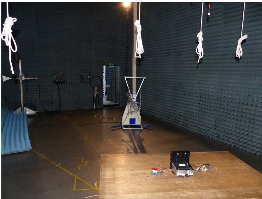
Photo 2: Test setup for radiated measurements (Enclosure, semi-anechoic chamber, 30 MHz to 1 GHz, intentional radiator §15, ANSI C63.10)
