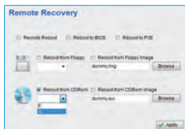
Remote Recovery: Mounts boot image or physical CD-Rom to target device
