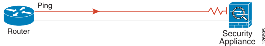
Figure 40-2 Ping Failure at Security Appliance Interface
