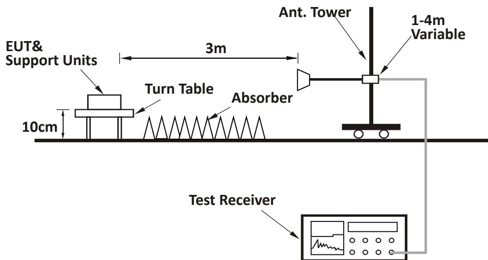
**TEST REPORT****7.4 Test Results of Radiated Emissions**
