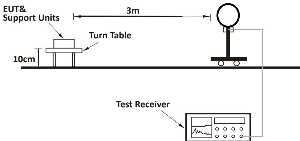
For Radiated emission 30MHz to 1GHz:
