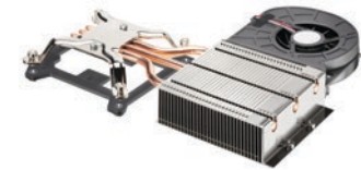
INTEL® THERMAL SOLUTION HTS1155LP
