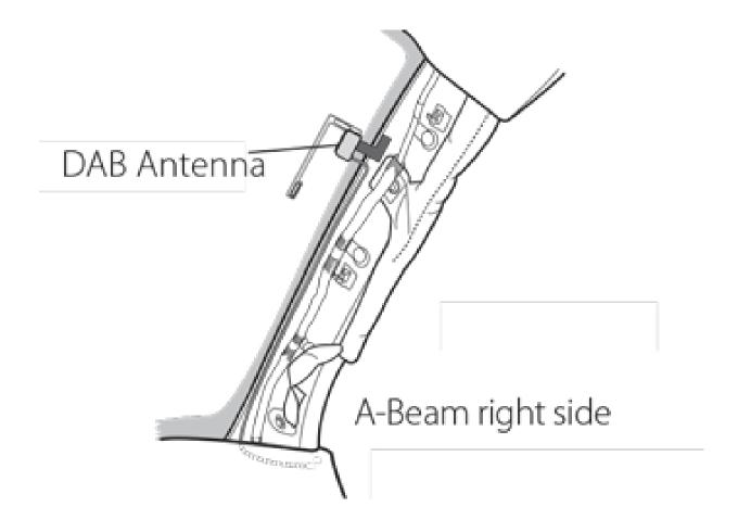
Do not attach the DAB antenna above heater wires, in a location which would obstruct the view of the driver, or in a location that would receive interference from metal. For your safety, do not run cables so that they interfere with operation of the vehicle, or through a location that would interfere with the function of the airbags.
