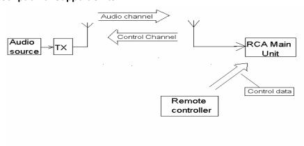
The MAIN UNIT(MU), USB DUNGLE(UD) and REMOTE CONTROLLER(RC) are a complete system. The system is based on wireless digital audio transfer from an audio source to MAIN UNIT, and REMOTE CONTROLLER can control MAIN UNIT by radio. It is noted that the communication between USB DUNGLE and MAIN UNIT are based on half-duplex transmission, MAIN UNIT and REMOTE CONTROLLER are base on simplex transmission.
