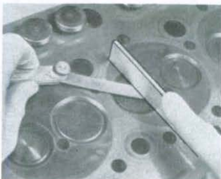
Fig. 63—A straightedge and feeler gage can be used as shown to determine how far valves are recessed.
