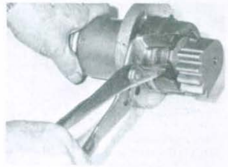
Fig. 7—The snap ring must be removed as shown before pitman shaft can be removed from housing.
