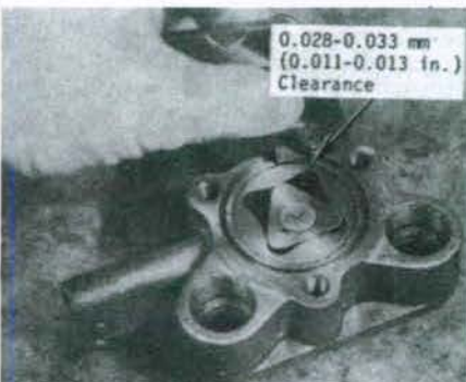
Fig. 80—Clearance between outer rotor and pump body can be measured as shown.
