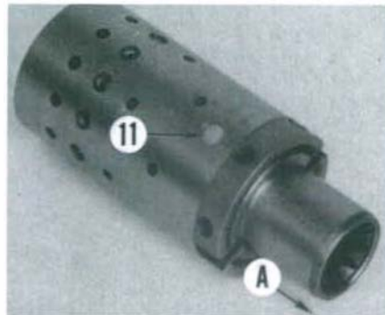
Fig. 25—View of control spool end sleeve assembly. Teflon discs (11) cover outer ends of internal pin. Withdraw spool from sleeve in direction of arrow (A).
