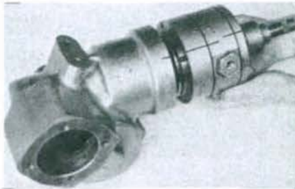
Fig. 15—Align scribe marks made prior to disassembly when assembling control valve, steering shaft, piston and rack assembly.
