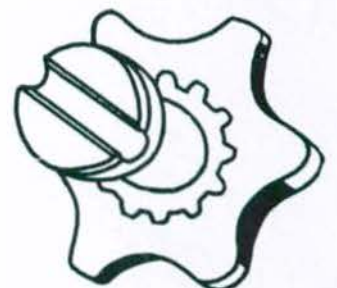
Fig. 26—When properly assembled, slot in end of drive link must align with valley of inner gear as shown to provide correct valve timing.
