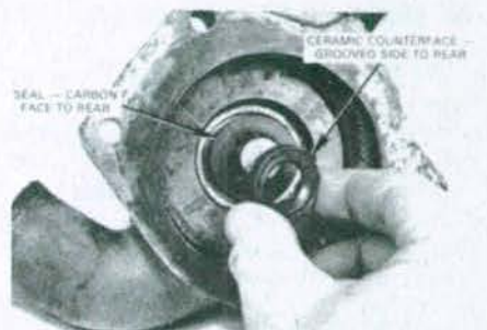
Fig. 83—Install front part of seal with carbon face toward rear. The ceramic counterface should be installed with grooved side toward rear.
