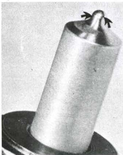
Fig. 88—Nozzle holes (arrows) are not located an equal distance from nozzle tip.
