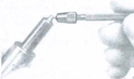
Fig. 91—Clean spray holes in nozzle tip using a pin vise and correct size cleaning wire. Refer to text.
