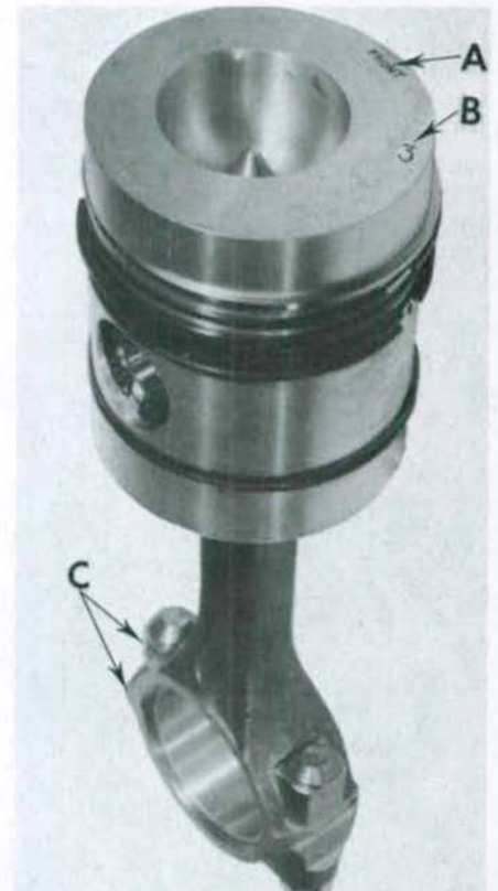
Fig. 71—Assemble rod and piston units as shown. A. FRONT or F mark B. Cylinder number C. Connecting rod correlation marks
