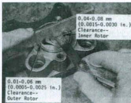
Fig. 81—Use a straightedge and feeler gage to measure end clearance between top of rotors and machined surface of pump body.
