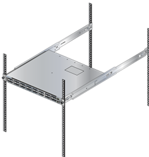
Figure 3-12: Attaching the Switch to the Rack Posts
