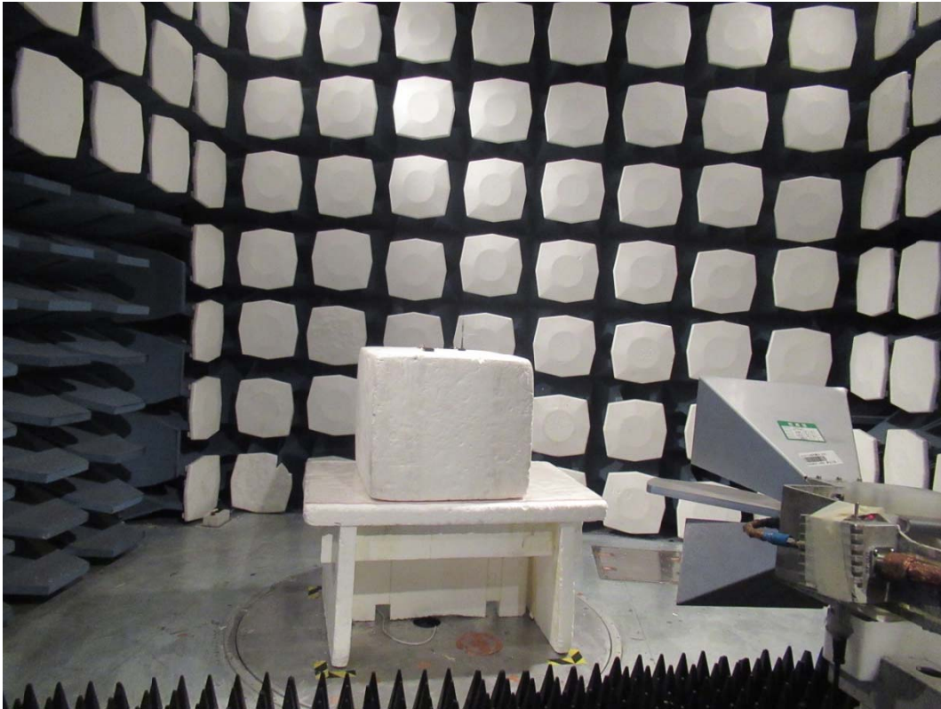
Picture 1: Radiated Spurious Emissions Test setup
