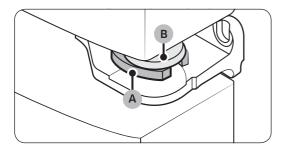
2. Insert a suitable-sized snap ring (A) between the door grommet (B) and the hinge as shown.
