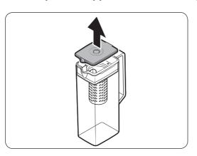
**1.** Grasp a handle groove of the **lid**, and then pull up to remove.
