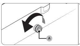
Open the door that is closer to the main body than the others. Then, turn the adjustment dial (A) counterclockwise until the gap becomes even with the others.
