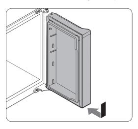
**1.** Insert the freezer door into the bottom hinge while pushing the freezer door in the direction of the arrow.
