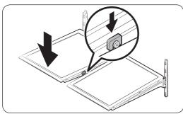
To remove a shelf, fully open the corresponding door. Hold the front of the shelf, and then gently lift up and pull out.
