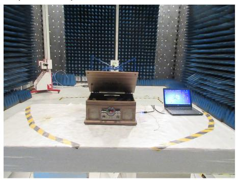
Photograph 2: Set-up for Radiated Spurious Emission, above 1GHz
