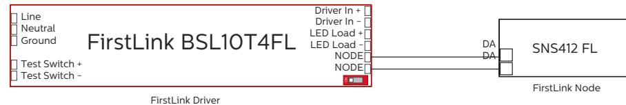
\* Wiring diagram for a BSL10T4FL shown. Other drivers might have different wiring diagrams. Consult datasheet of the driver for applicable wiring diagram.
