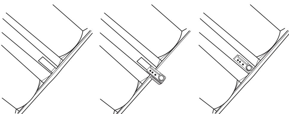
Mounting in a cut-out with mounting bracket
