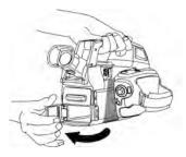
3. Push the battery into the battery compartment.
