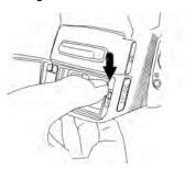
4. Pull out the battery from the battery compartment.
