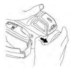
2. Rotate the infrared lens counter-clockwise 30° (looking at the front of the lens).
