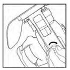
**Note** When you remove the heatshield you must reset the external optics transmission to 1.0.
