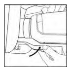
5. Mount the aluminum frame by tightening the mounting screw.
