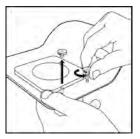
2. Push the aluminum frame onto the screws.
