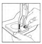
4. Align the aluminum frame to the mounting interface on the bottom side of the camera body. The aluminum frame has an alignment peg that should fit in a hole on the camera body.
