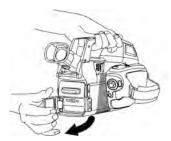
3. Push the release lever for the battery downward.
