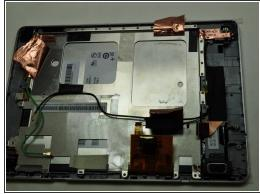
Lift the three copper foils from the plate.
