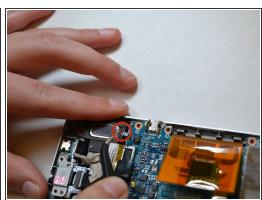
Disconnect all cords, wires, and resistors from the motherboard using tweezers.
