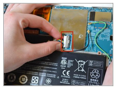
Pinch the sides of the white resistor to safely remove it without damaging it or yourself.
