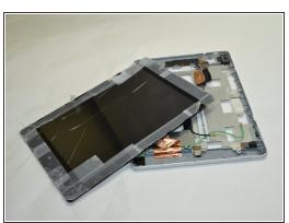
While holding the side of the screen, press the metal plates behind the device to pop the screen out.
