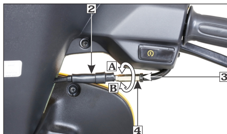
(2) Boot (3) Lock nut (4) Adjuster (A) Decrease free play (B) Increase free play
