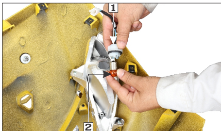
(1) Bulb holder (2) Front turn signal bulb
