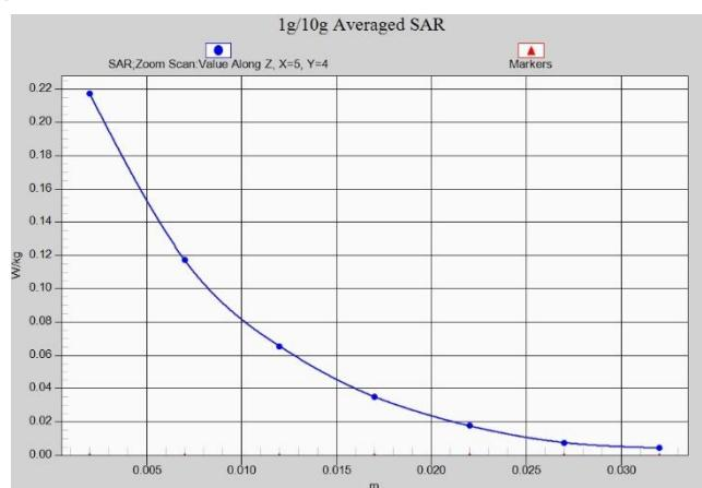
**Fig.A.24- 1 Z-Scan at power reference point (Wifi2450)**
