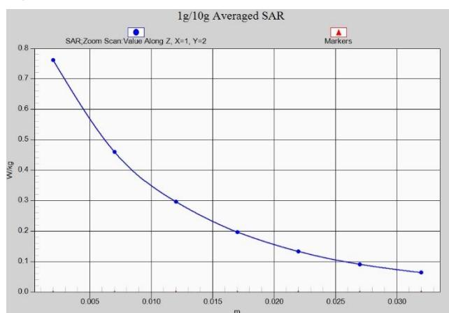
**Fig.A.6- 1 Z-Scan at power reference point (W850)**
