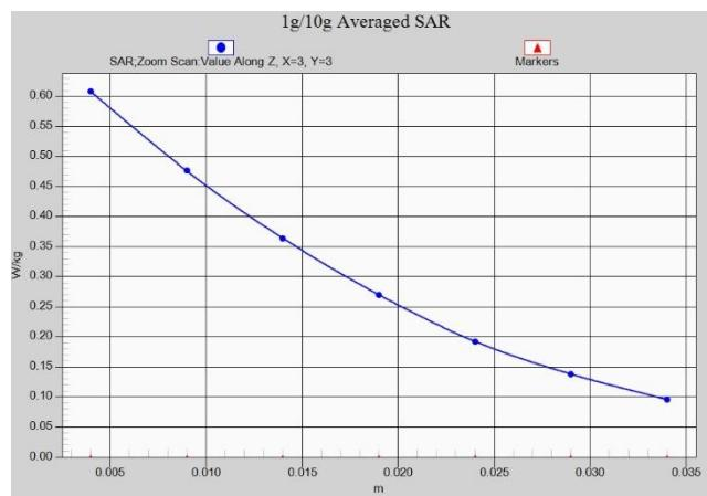
**Fig.A.3- 1 Z-Scan at power reference point (PCS1900)**
