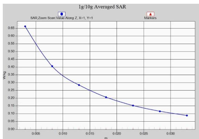
**Fig.A.5- 1 Z-Scan at power reference point (W850)**
