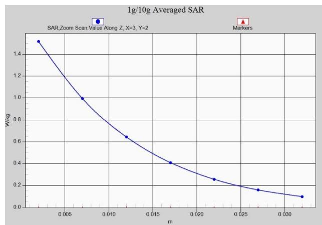
**Fig.A.11- 1 Z-Scan at power reference point (W1900)**
