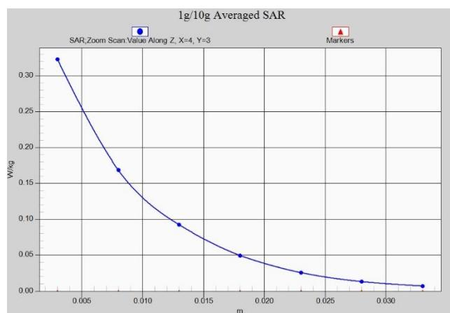
**Fig.A.23- 1 Z-Scan at power reference point (Wifi2450)**
