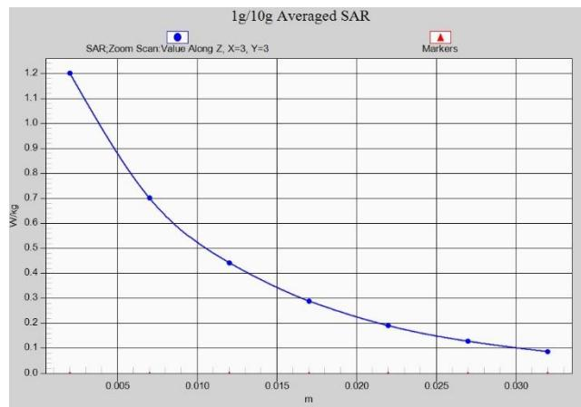
**Fig.A.2- 1 Z-Scan at power reference point (GSM850)**
