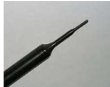
Picture C.2Near-field Probe
