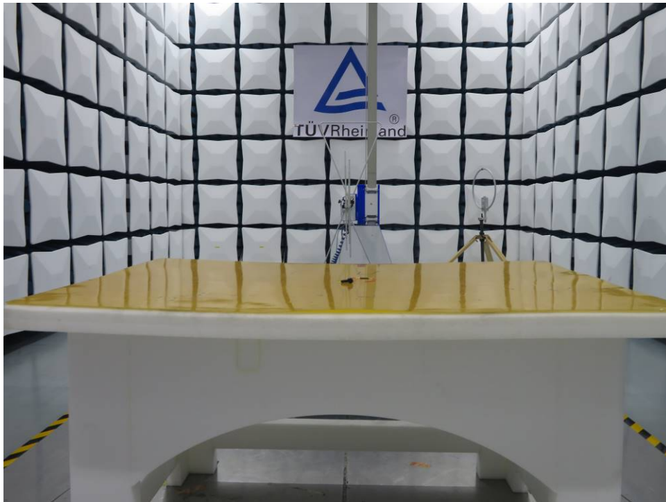
Photograph 1: Set-up for Radiated Spurious Emission, Below 1GHz
