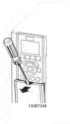
Illustration 5.37: Access to control terminals for A2, A3, B3, B4, C3 and C4 enclosures
